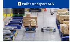
Pallets full of incoming products are transported to the intake facility of the automated warehouse, increasing work efficiency by reducing the need for workers.
