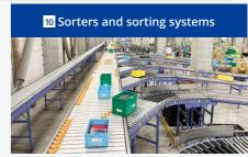
Sorters are controlled by systems to divide products by their outgoing direction and delivery carrier.
