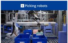
These arm-type robots use 3D-image recognition to automatically generate a movement plan to identify and pick out 2,000 varieties of products. 2 centers
